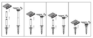
(2) Insert the assembled light into the ground vertically.
