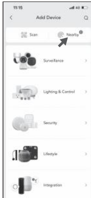
2 Choose the device what you find in 'Nearby' (PS: You must open the Bluetooth and Location Services. If you still can not fine the device in 'Nearby', Try to reset the device: Long press the button for more than 10S to enter flash mode.)
