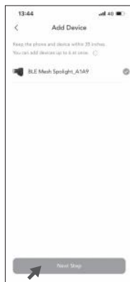
2 Choose the device what you find in 'Nearby' PS: You must open the Bluetooth and Location Services. If you still can not find the device in 'Nearby', Try to reset the device: Long press the button for more than 10S to enter flash mode.
